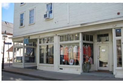
The commercial building at 78-80 Thames Street has frame bulkheads which could be protected by flood shield panels.
