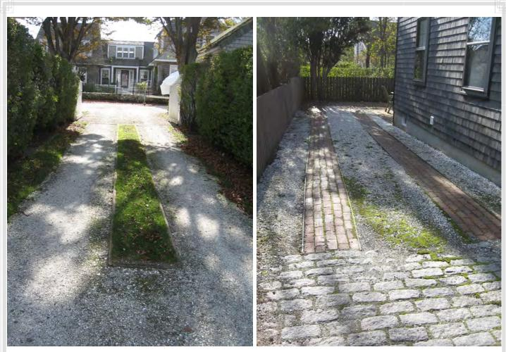
**YES:** Property owners are encouraged to use permeable materials for driveways such as gravel instead of hard surfaces like concrete or asphalt (left). Another approach is to only hard surface the driveway "ribbons" as shown at right (Nantucket, Massachusetts).
