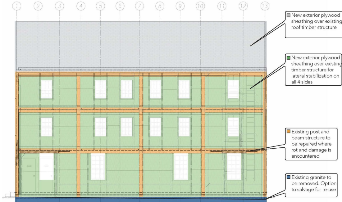
Preliminary Structural Repairs
