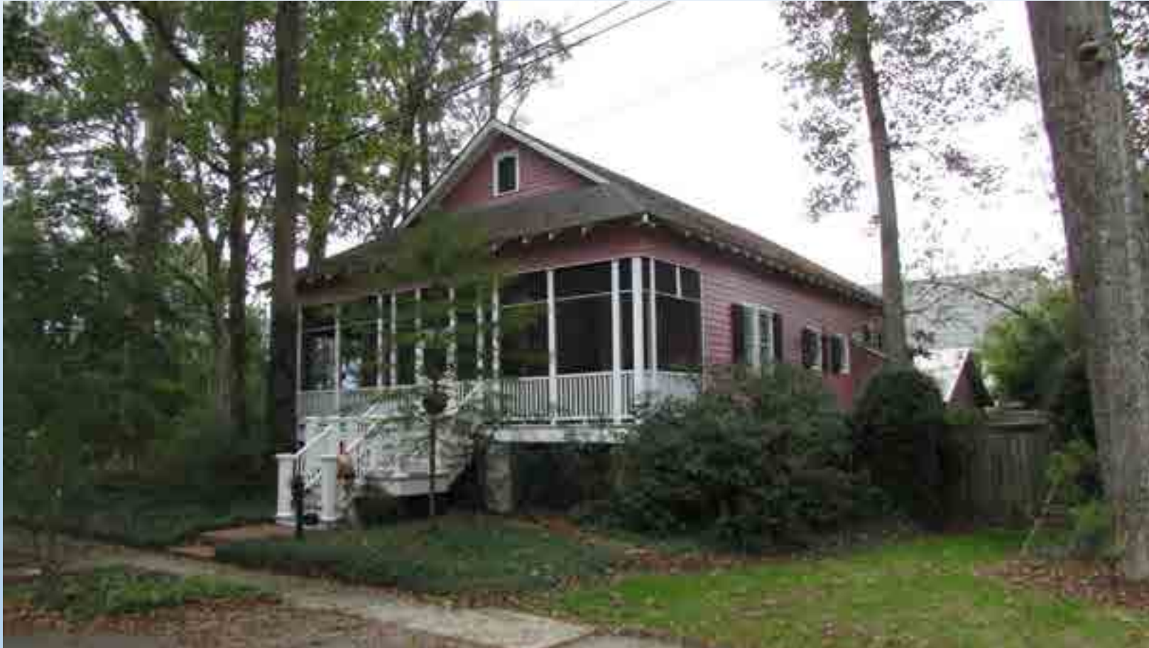
LOW ELEVATION WITH OPEN FOUNDATION
